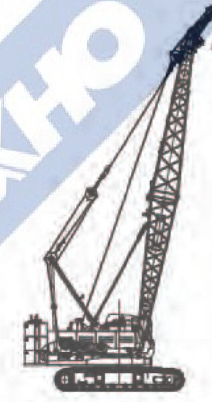
臂端单滑轮工况 (主臂不带吊钩) Boom single pulley mode (without hook block)
