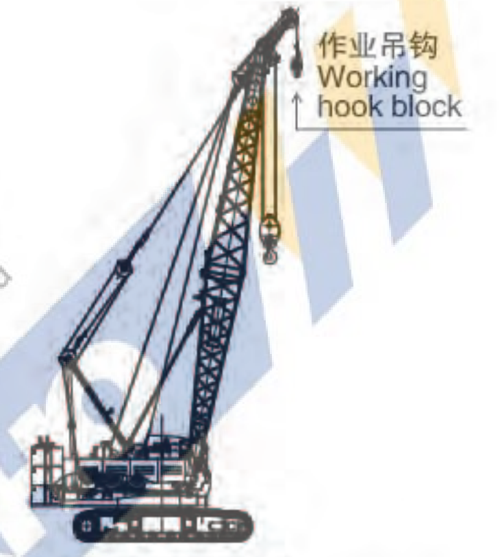
臂端单滑轮工况 (主臂带吊钩) (选配) Boom single pulley mode (with hook block) (Optional)
