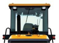
Full-view rear window, high mounted rear lamp and equipment for reverse alarm provide good vision and safe reversing.
