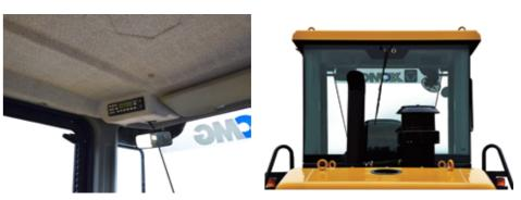
Fully-covered exquisite interiors, processed cab and hood for damping noise reduction, reduce the noise by over 6dB and provide best operation environment.
