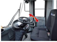
Luxurious shock-absorption seat and steering gear adjustable at will cater to operation habits and operation requirements of operators with different figures.
